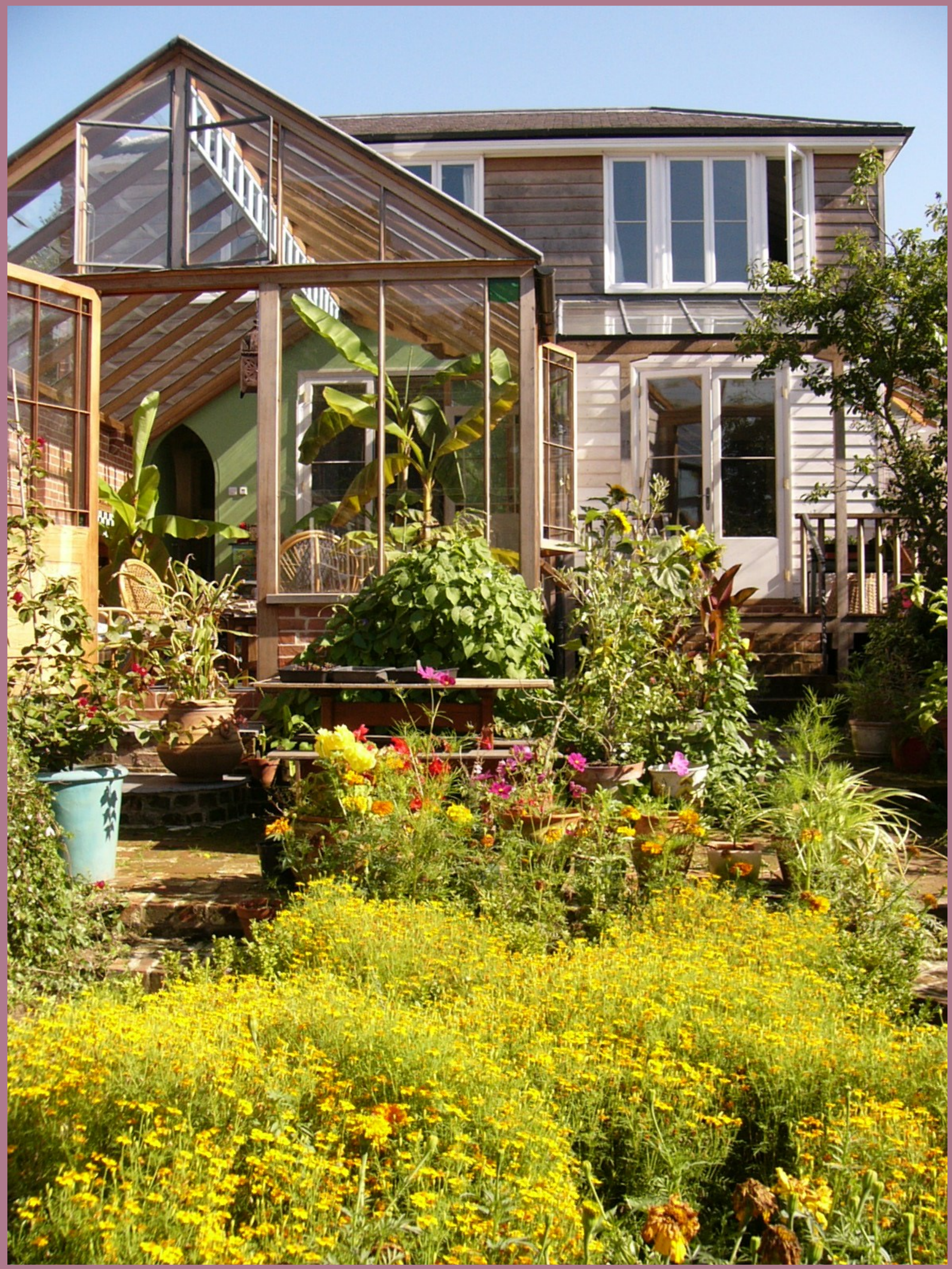
New conservatory with black limestone floor and cedar structure - the brick wall on the right is highly insulated for thermal mass
